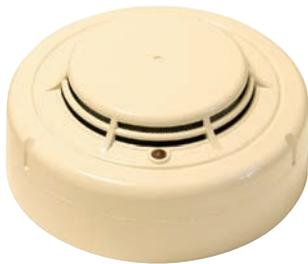
The SD-851E forms part of the processor enhanced detection series of conventional detectors. It incorporates an optical chamber which is continually monitored by an on board processor which uses algorithms developed specifically for the unit. An alarm signal is only enabled in the detector once the processor is satisfied that an incipient fire has been detected thereby reducing the incidence of nuisance alarms.
