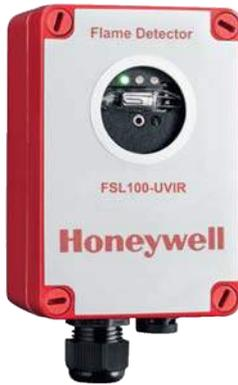
Analyses the flame flicker frequency to improve false alarm rejection, the dual sensing methodology enable the effectively detection of a wide range of hydrocarbon and non-hydrocarbon fires. It offers also a good resistance against direct and reflected sunlight and artificial light, arcs and electric discharge.
