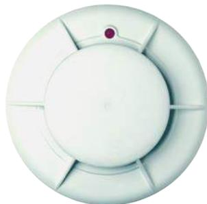
The ECO1003 photoelectric smoke detector uses a state of the art optical chamber combined with an application specific integrated circuit (ASIC) to provide quick and accurate detection of fires. A combination of the unique chamber design and other technically advanced features will significantly extend the service intervals before the cleaning of the detector becomes necessary.
