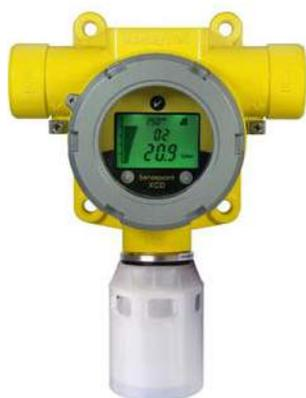
The standard XCD detector is supplied including one of three types of plug-in stainless steel sensor. These sensors simply plug into the socket at the bottom of the transmitter and the transmitter recognizes the sensor type and automatically configures itself accordingly.
