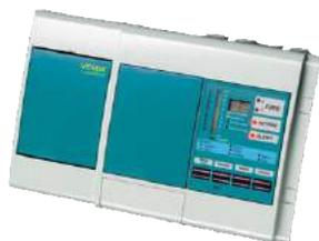
As VLP-400, but with a standard display module for reading the actual status of the detector including alarm levels and system faults. The display is equipped with 4 push buttons for Mode, Mute, Reset and Isolate.
