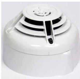
The NRX-TDIFF heat sensor is a battery operated RF device designed for use with the NRXI-GATE radio gateway. It contains a wireless transceiver and runs on a NOTIFIER intelligent fire system (using a compatible proprietary communication protocol). The NRX-TDIFF provides 58°C rate-of-rise (10°C/minute) temperature sensing (A1R).
