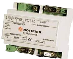
This gateway allows to integrate the NOTIFIER panels through MODBUS protocol. The gateway acts as a MODBUS slave device. Commands toward the panel are allowed (conventional zones). Immediate response, operation based on events. DIN rail, wall or desktop mounting. Power from 9 to 30VDC (Power supply included).
