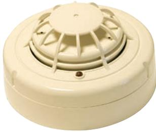
The FD-851RE forms part of the processor enhanced detection series of conventional detectors. The FD-851RE thermal detector incorporates the latest in thermal element technology, the detector provides efficient and accurate detection of fires, especially in environments such as boiler houses or kitchens where smoke detectors are inappropriate due to the high level of airborne contamination.
