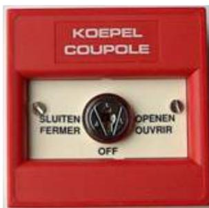
Key switch as external priority control with open, close and neutral position. The key switch contains electronics to connect this three position switch with only two, polarity independent wires, to the Sahep panel. The connection is supervised with a built in end of line resistor. Maximum one SAHEP-PRIOR can be added on a Sahep panel.
