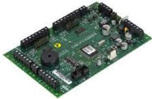
Compatible with NF30/50 and NF3000 Panels. 16 outputs on board and up to 9 expansion boards (020-742) can be added (drive led's or relays), giving max. of 160 outputs.
