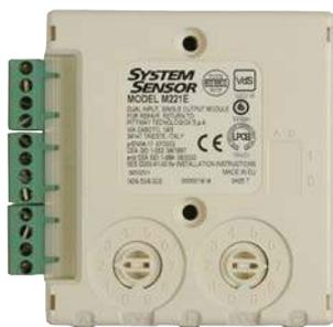
In addition the M721 dual input, single relay output module, as well as providing two supervised inputs also provides a single change over relay output rated at 2A @30VDC.
