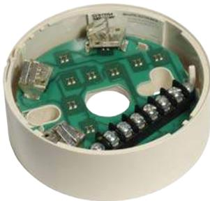
Standard base with heater, compatible with the NFXI series. Raises the temperature of the detector to avoid condensation in the detection room.
