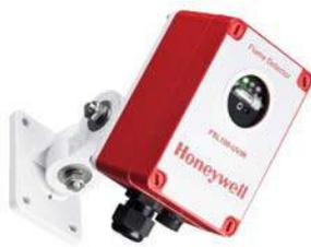
The FSL100 series consists of UV, UV/IR and IR3 flame detectors utilising sophisticated sensing and signal analysis to detect fire quickly while also rejecting false alarms. THE FSL100 is designed to work in tough indoor/outdoor environments, as well as potentially explosive atmospheres.
