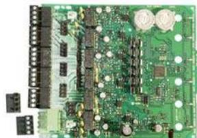
The SC-6 six way supervised sounder output module is intended for use in an intelligent alarm system. Each module is intended for switching applications involving DC which require wiring supervision. A common SLC input is used for all modules. Each module has its own address. A pair of rotary code switches is used to set the address of the first module from 01 to 94. The remaining modules are automatically assigned to the next five higher addresses.
