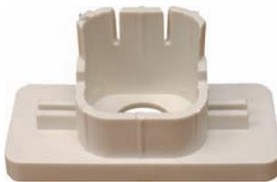
The mounting adapter is used for the quick and secure attachment of bases of the NFXI, SD800 and ECO detector series to suspended ceiling systems. It saves the usage of special hollow cavity fasteners, since the mounting screws of the bases are screwed directly into the slots of the mounting adapter. The mounting adapter offers additional advantages in the fixing of the cables, rigid/flexible cable inlays and threaded cable connections.
