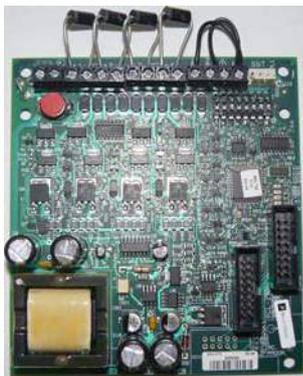
Provides 4 monitored circuits with provision for external PSU and 2 digital inputs.
