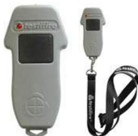
The remote control for Testifire is required for situations where the IR test beam of Testifire that triggers or stops a test is not broken by a physical presence. Typical situations are the sampling ports of aspirating detection systems or detectors with 'virtual chambers'. The Testifire 25 is then used to initiate the test procedure.
