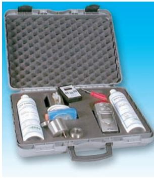
All SENSITRON gas detectors are factory calibrated prior to despatch. In order to fulfil the EN60079–17:2003, detectors have to undergo periodical operational testing, each three to six months according to the plant’s risk assessment. Test results are to be recorded into a suitable book to be shown to the Authority in case of inspection.
