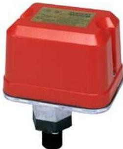
EPS40 Series switches are designed for use in wet, dry, deluge, and pre-action automatic sprinkler systems to indicate a discharge from a sprinkler. The EPS40-1 has a single SPDT switch. The EPS40 Series feature field adjustable pressure sensitivity to provide an alarm response between 10 and 100 psi. The EPS40-1 is factory set to respond at 30 psi at decreasing pressure.
