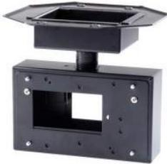
Ceiling pendant mount for use with F5000, F50/100, prism and 5000-005 universal bracket. Includes universal mounting plate. Does not include universal mounting brackets or 5000 detectors. Ceiling pendant mount comes with a 1" x 12" long threaded nipple. Contractor shall provide other nipple lengths as required.
