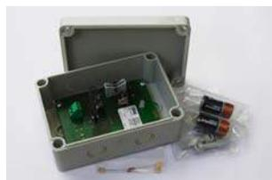
The wireless monitored input module allows the switched on/off status of an external device to be transmitted to the control panel through translator / expander devices.
