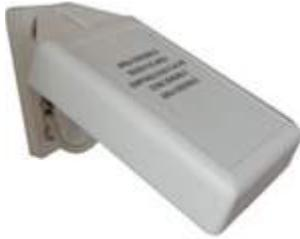
The SAHEP-RD rain detector functions with a capacitive sensor. So rain is detected in a capacitive way. In a capacitive rain sensor no external PCB traces are visible. These traces are sensitive for oxidation. This rain detector is compatible with the WRD1. A mounting bracket is included.
