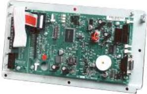
Compatible with NF30/50 and NF3000 Panels. Mimic control PCA Kit. Supports up to 8 Mimic Drivers. Requires ext. 24VDC Power source and min. one 020-574. Use the mimic driver configuration tool kit (020-613). For use with "network zones".
