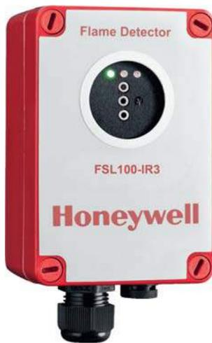
Analyses the flame flicker frequency to improve false alarm rejection, it is particularly suited to liquid hydrocarbon and dirty fire that emit large amount of smoke. It offers also a good resistance against direct and reflected sunlight and artificial light, arcs and electric discharge.
