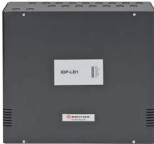
The Loop Booster has been designed to provide extra power to a loop to power additional loop powered devices, especially high current drawing 'alarm' devices such as loop powered sounders and strobes. As an intelligent device a number of loop boosters can be added to a loop within the normal intelligent range (01 to 99). It is recommended that no more than 2 loop boosters be added to any particular loop.
