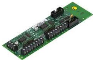
Provides 16 LED's or relays outputs. Up to 9 expansion boards can be daisy chained. Requires 020-741 IDR-CM Mimic main board.
