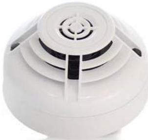
The NFXI-TFIX58 is fixed temperature intelligent sensors employing low mass thermistors and microprocessor technology for fast response and linear temperature sensing. Their linear response allows these sensors to be used to signal temperatures over the range of 58°C (Class A1S).
