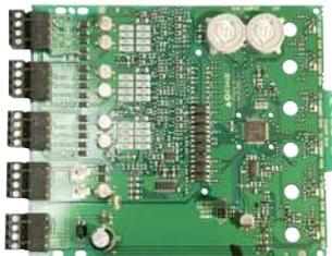
The CZ-6 way zone interface module is intended for use in an intelligent alarm system. Each input module provides an interface between the intelligent alarm system and a conventional alarm system loop. A common SLC input is used for all modules, and the initiating device loops share a common supervisory supply and ground. Otherwise, each monitor operates independently from the others. Requires a separate reset.
