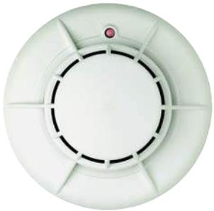
The ECO1002 multi-criteria detector uses a state of the art optical chamber and a class A1R thermal element combined with a microprocessor, running sophisticated algorithms to provide quick and accurate detection of fires.
