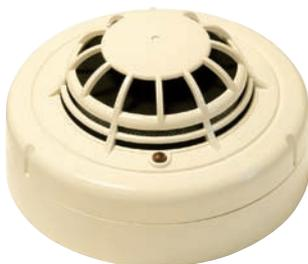
The SD-851TE photoelectric smoke/ thermal detector incorporates an optical chamber and a thermal element, which in turn are continually monitored by an on board processor by using algorithms developed specifically for the unit. An alarm signal is only enabled in the detector once the processor is satisfied that an incipient fire has been detected.
