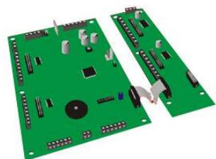
Compatible with NF30/50 and NF3000 Panels. 16 outputs on board and up to 9 expansion boards (020-742) can be added (drive led's or relays), giving max. of 160 outputs. 5 led outputs (Power ok, Test, Gen. Fault, Disablement & Fire) and 6 inputs (Key switch, Evacuate, Mute Buzzer, Silence sounders Lamp test & Reset). Requires ext. 24VDC Power source. For use with "local zones".
