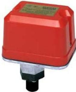
EPS10 Series switches are designed for use in wet, dry, deluge, and pre-action automatic sprinkler systems to indicate a discharge from a sprinkler. The EPS10-1 has a single SPDT switch. The EPS10 Series features field adjustable pressure sensitivity to provide an alarm response between 4 and 20 psi. It is factory set to respond at 4 – 8 psi on rising or falling pressure. The EPS10 Series switches are NEMA 4 rated.
