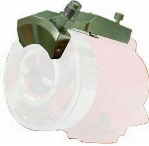
The air shield enables the connection of a compressed air line to provide an 'air curtain' that helps avoid accumulation of dirt on the detector window thereby reducing maintenance need and frequency in polluted or dirty environments.
