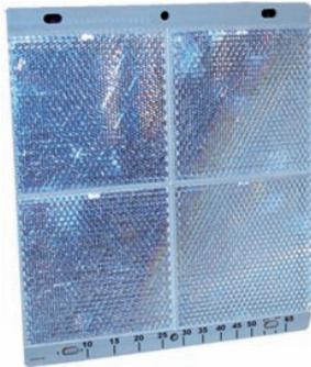
The BEAM-LRK kit contains 3 reflectors (200mm x 230mm). In combination with the short range reflector supplied with the beam, the 4 reflectors mounted in square form one big reflector surface which extends the beam range over 70m, up to a maximum distance of 100m.
