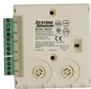
The M701 control module provides a monitored single output circuit for use with polarised loads (sounder circuit) which requires a suitable power source (7VDC - 30VDC) for the connected load. Alternatively the same device may be placed in to an unsupervised mode which can then be used to control any switched load up to 2A @ 30VDC.
