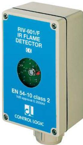
The IR flame detector model RIV-601P/F is an electronic optical fire detecting device which responds immediately to the thermal infrared radiation emitted by fire and is turned to the flickering frequency of the flame to ignore sun and lamp light.
