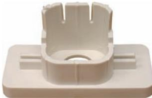
The mounting adapter is used for the quick and secure attachment of bases of the NFXI, SD800 and ECO detector series to suspended ceiling systems. It saves the usage of special hollow cavity fasteners, since the mounting screws of the bases are screwed directly into the slots of the mounting adapter. The mounting adapter offers additional advantages in the fixing of the cables, rigid/flexible cable inlays and threaded cable connections.
