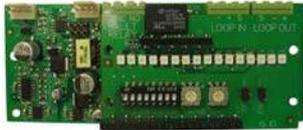
Communication card to transmit the information of the extinguishing control panel to the intelligent NF30/50 or NF3000.
