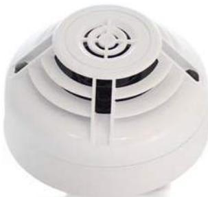
The NFXI-TFIX78 is fixed temperature intelligent sensors employing low mass thermistors and microprocessor technology for fast response and linear temperature sensing. Their linear response allows these sensors to be used to signal temperatures of 78°C (Class BS).
