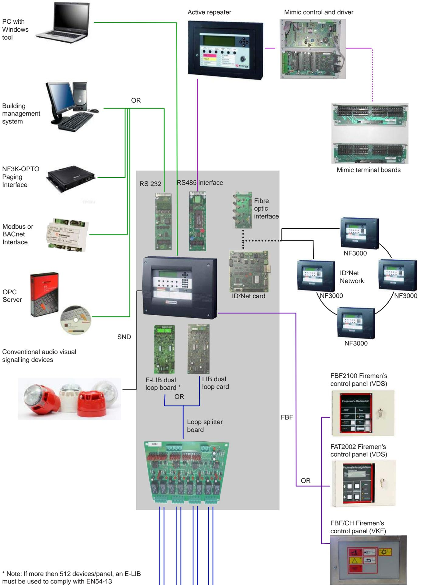
\* Note: If more than 512 devices/panel, an E-LIB must be used to comply with EN54-13
