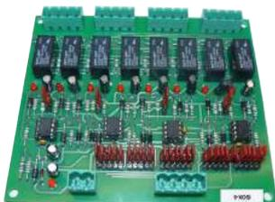
Transforms 1 intelligent loop into 4 closed and isolated sub-loops.
