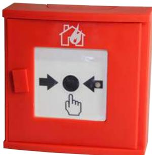
The NRX-DKM radio call point is a battery operated RF device designed for use with the NRXI-GATE radio gateway running on a NOTIFIER intelligent fire system (using a compatible proprietary communication protocol).
