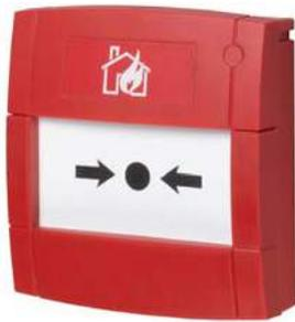
The MCP1A range are Manual Call Points (MCP), both with a 470 Ohm resistor and normally open contact, complete with Plexi. The MCP1A-R470FF-01 is designed for flush mounting. The call points are designed to provide a manual alarm interface to conventional fire alarm control panels and are supplied in the standard red colour.
