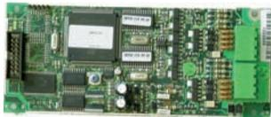
Includes PCB for additional 2 loops with on board standby microprocessor, and plug in cable connector. Max. three modules per panel. Only required where total number of input devices controlled by panel main microprocessor exceeds the EN54 limitation of 512. E-LIB may be mixed with standard LIBs in the same panel.
