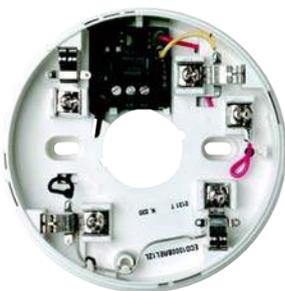
Interface for 24V system that requires an external contact. The detector stays in alarm until the removing of its supply voltage. A break-off tab allows the base to be connected to fire control panels. This tab should be broken when there is little current flow or no current limiting resistor such as when used as a 24V stand-alone system.
