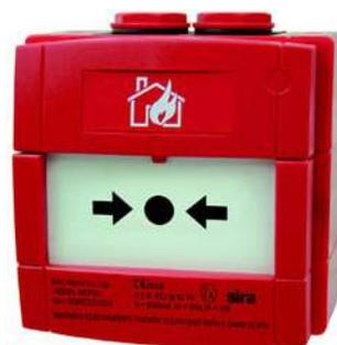
Includes flexible element, surface mounting box, a normally open contact (max. 30VDC) and 470R monitoring resistor.
