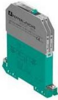
This surge protection barrier limits induced transients of different origin (e.g. lightning stroke, switching impulse, etc.). This is achieved by diverting the transient current to ground and limiting the signal line voltage to a safe level for the duration of the surge. It also protects instruments such as zener barriers.
