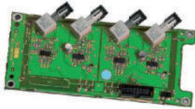
The fibre optic interface PCB plugs directly into the NGM via a ribbon cable. Two ports are available for fibre optic communication (left & right channel).
