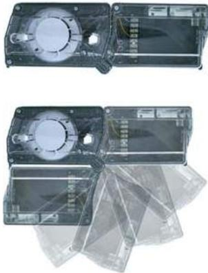
The DNRE Air Duct Smoke Detector uses photoelectric technology for the detection of smoke. This detection method, when combined with an efficient housing design, samples air passing through the duct and allows detection of a developing hazardous condition.
