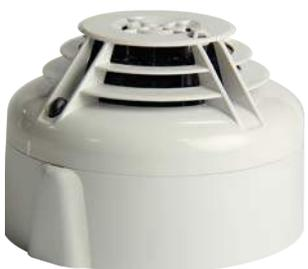
The NRX-SMT3 radio sensor is a battery operated RF device designed for use with the NRXI-GATE radio gateway. It contains a wireless transceiver and runs on a NOTIFIER intelligent fire system (using a compatible proprietary communication protocol). It is a multi-criteria smoke and heat detector (58°C Rate-of-Rise). An infrared sensor adds further detection ability and increased immunity to false alarms. The sensor plugs into the B501RF wireless sensor base (not included).
